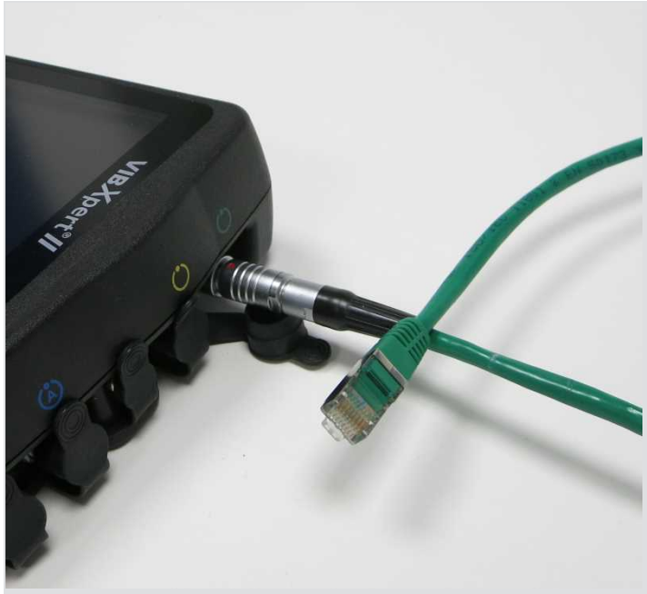
Ethernet cable connected to VIBXPART II
