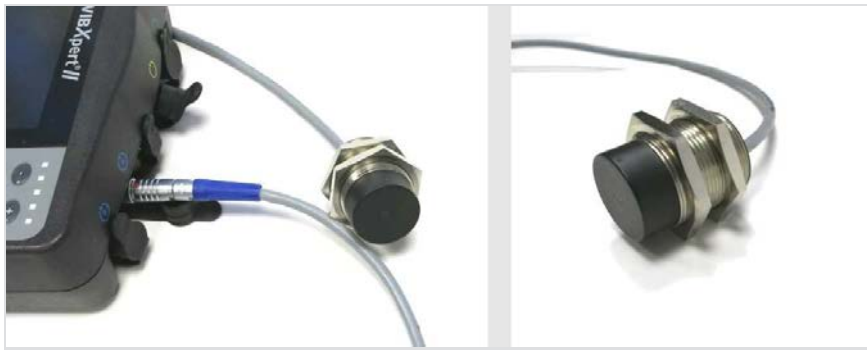
Displacement sensor connected to VIBXPART II
