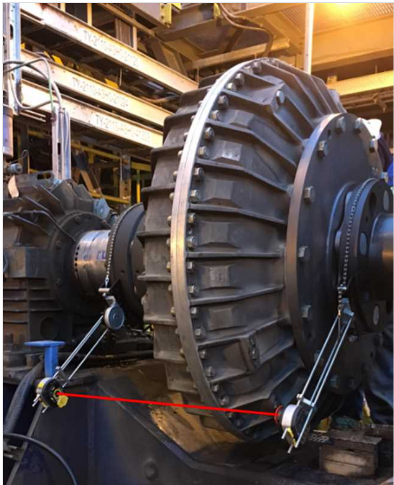
Chain-type bracket for large diameter, ALI 2.460
