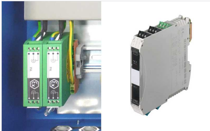
Limiting devices for CLD accelerometers (installed, left) and for VIBROTECTOR (right)
