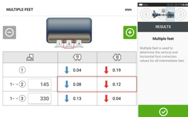
The screenshot shows the 'MULTIPLE FEET' interface with a table of correction values and a 'RESULTS' panel. The table has three columns: a column for foot numbers, a column for vertical correction (blue arrows), and a column for horizontal correction (red arrows). The second row is highlighted with a red border, indicating the current selection.
