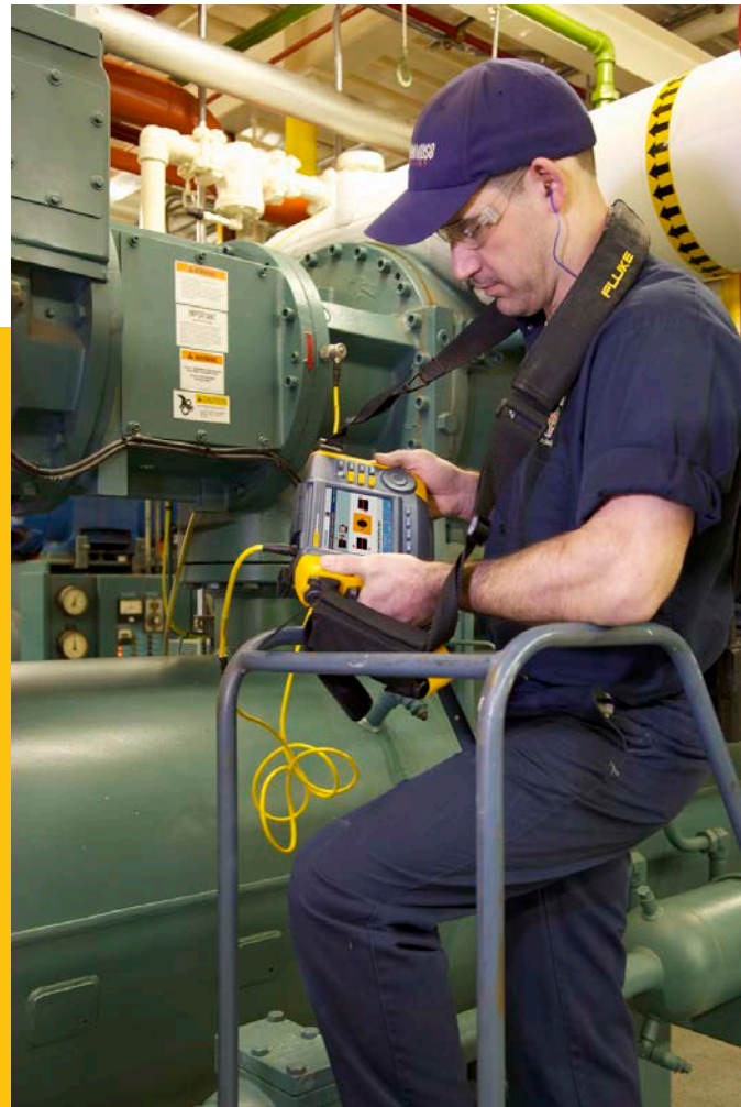
At Alpenrose Dairy regular vibration analysis provides data for trend analysis used in proactive maintenance.
