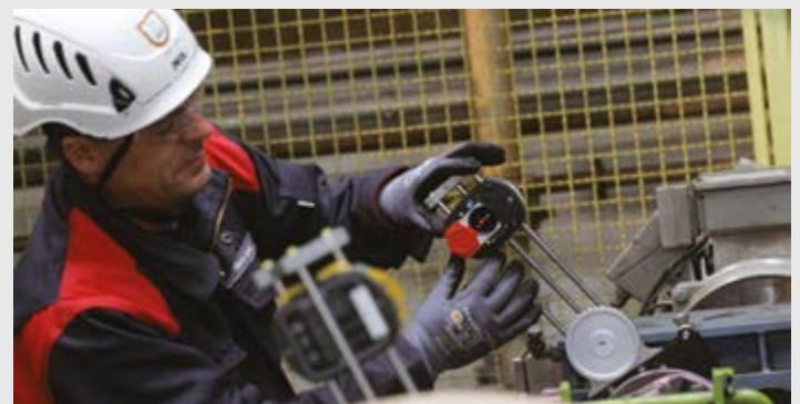
Laser-optical alignment of an installed cardan shaft
