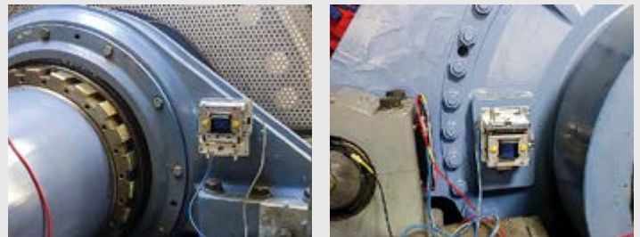
Arrangement for online recording of thermal deformations of the main bearing and the main gearbox in relation to each other
